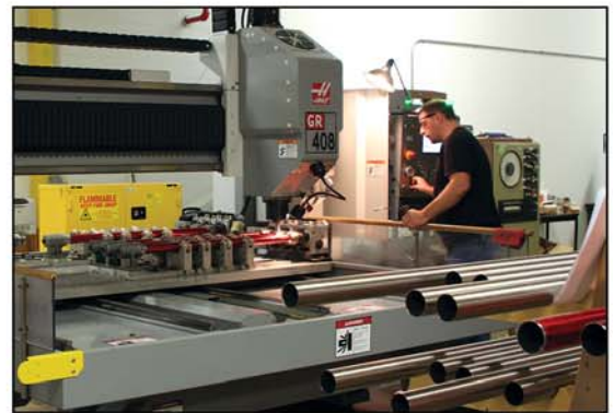
Haas Gantry Router Machine
